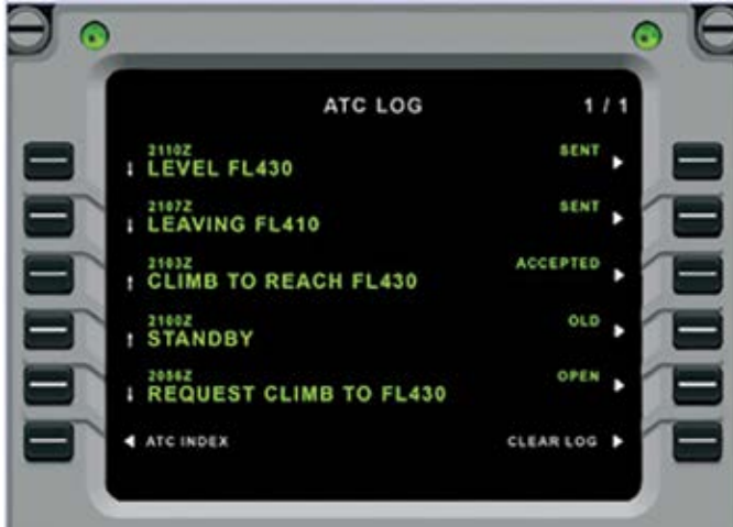
Figure 1: Sample ATC Communications using Protected ATS Datalink.
