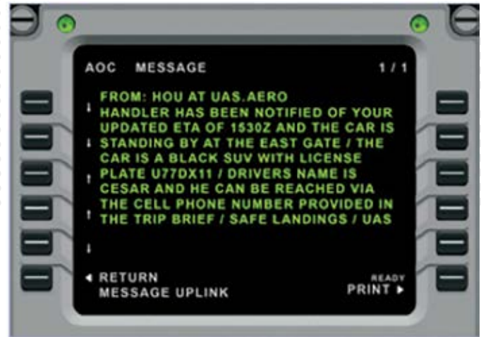
Figure 2: Sample Message using Unprotected AOC Free-Text.
